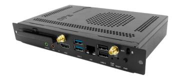
7th Generation Intel® Core™ i5 Processor. The Intel® Open Pluggable Specification (OPS) PC is designed to turn your Avocor Interactive Display into a big-screen all-in one touch PC
